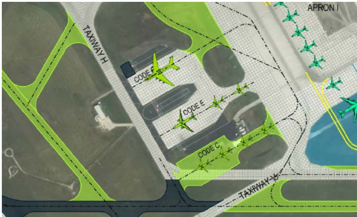
Figure 7-1: Proposed Expansion of the Central De-icing Facility
